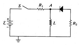
94. In the circuit shown above,  $R_2 = 3R_1$  and the battery of emf E has negligible internal resistance. The resistance of the diode when it allows current to pass through it is also negligible. At time t = 0, the switch S is closed and the currents and voltages are allowed to reach their asymptotic values. Then at time  $t_1$ , the switch is opened. Which of the following curves most nearly represents the potential at point A as a function of time t?
