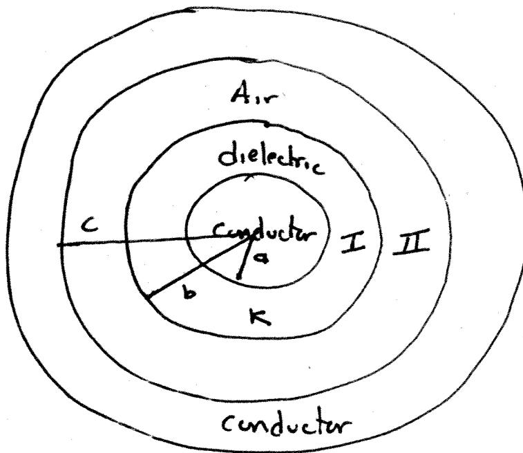
Note, dielectric does not completely space between conductors so  $C_k \neq kC_0$ .
