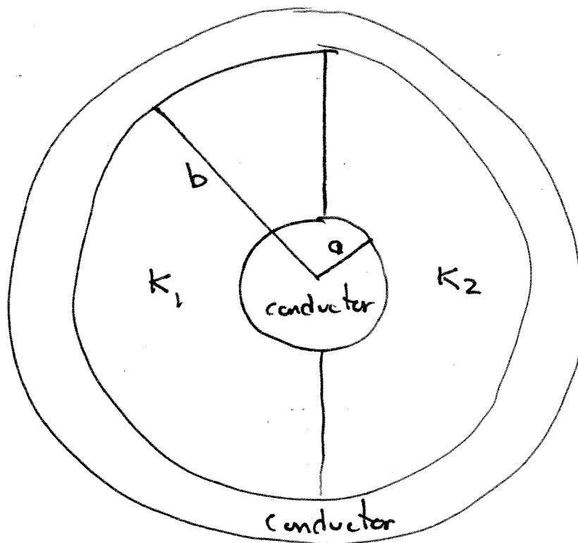
Place  $+Q$  on inner conductor,  $-Q$  on outer.
