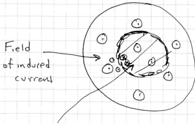
Flux increasing out of the page, so induced current produces flux into the page, induced current must flow clockwise by RHR.
