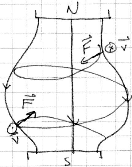
Field with gradient forces particles to center
