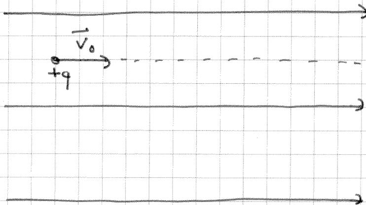
$$\vec{F}_m = q \vec{v} \times \vec{B} = q v_0 \hat{x} \times B_0 \hat{y} = 0$$
