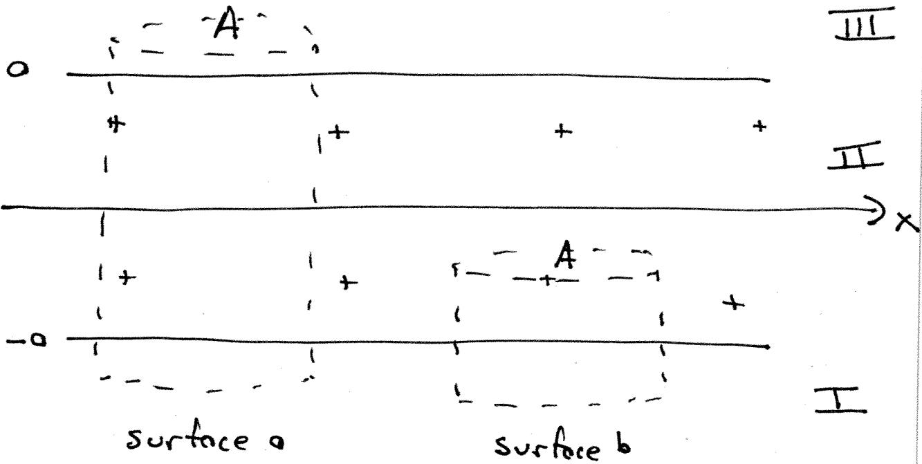
Surface o Apply Gauss' Law for Displacement
