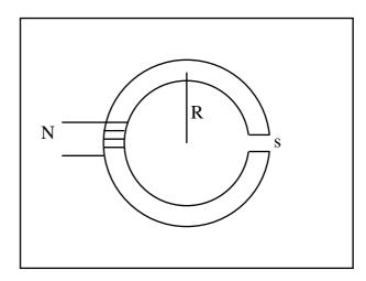
**E.9.2** Repeat problem E.9.1 where 1/10 the circumference of the iron is replaced with a permanent magnetic material with magnetization  $M = 10^5$  A/m. The permanent magnet produces a field in the same direction as the field produced by the wraps of wire.
