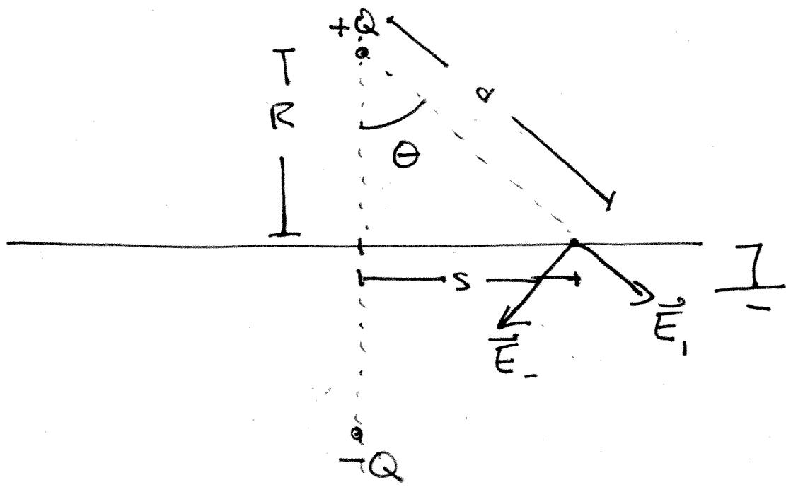
$$\text{At Plane, } \vec{E}_{\text{plane}} = \vec{E}_+ + \vec{E}_-$$
