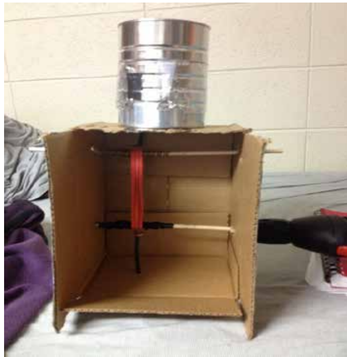
Figure 4: The frame of the machine was replaced with a box with the rollers running vertically above each other. The coffee can conductor is placed on the top of the machine and the hand drill motor it attached to the right side of the bottom roller.
