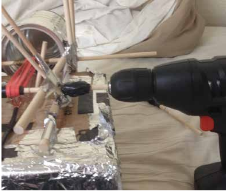
Figure 2: The high power drill is attached to the end of the vinyl roller to rotate the belt and cause a net charge.
