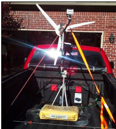
Figure 3: Turbine mounted in truck with camera setup for getting multimeter readings
