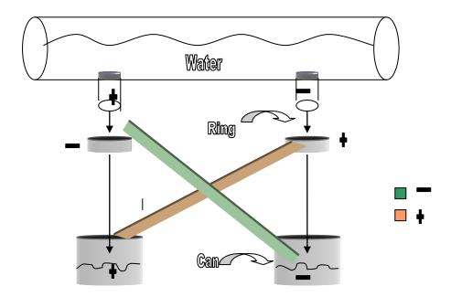
Naturally, some things will be slightly more charged than another. To go along with the drawn diagram, we will say that the bottom left can is slightly more positive than the right can. Therefore, the right can will posses a more negative charge. The right ring will possess a positive charge since it is connected to the positive can. This positive ring will attract the negatively charged ions by electrostatic induction. The negatively charged droplet will then fall from that ring
