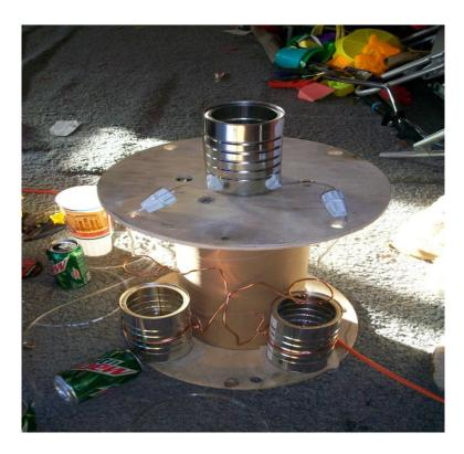
This picture demonstrates the final set up for the Lord Kelvin electrostatic water drop generator. The next step is to turn the water dripper on and see what happens. The following photo is a close up of the water dripping from the tubing through the copper wire and into the can below:
