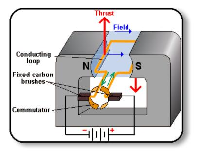
As the carbon brushes pass the gaps in the copper ring, the current is automatically switched, therefore keeping the rotational force in one direction. If the copper ring did not have the gaps the motor would rotate until it flip 180 degrees then the force would be in the opposite direction causing the motor to stop or reverse.
