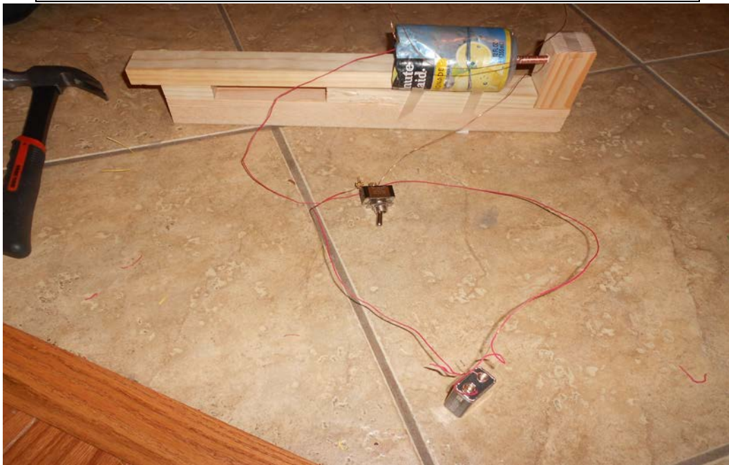
Figure 3: Initial construction using metal soup can of diameter 3.75 inches and one 9V alkaline battery
