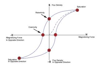
The curve above is referred to as a hysteresis loop and characterizes the relationship between a magnet and an applied field. When a magnetic field of strength  $\mathbf{H}$  is applied to a magnetic material, the individual atomic moments in the material contribute to the overall magnetic induction  $\mathbf{B}$  of the material.
