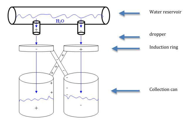
The Kelvin water dropper relies on two principles to operate. The first is electrostatic induction. This is defined as the distribution of electric charge on one material under the influence of a near by object with an electric charge (Britannica). The second principle is that of positive feedback. This is simply any effect that causes more of itself.
