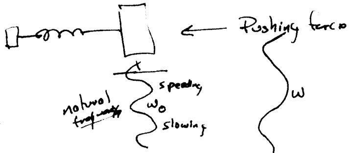
Sometimes if pushing force not in tune, energy is removed instead of added. If force is in turn, energy is always added. In a SHO no energy is lost so BANG.
