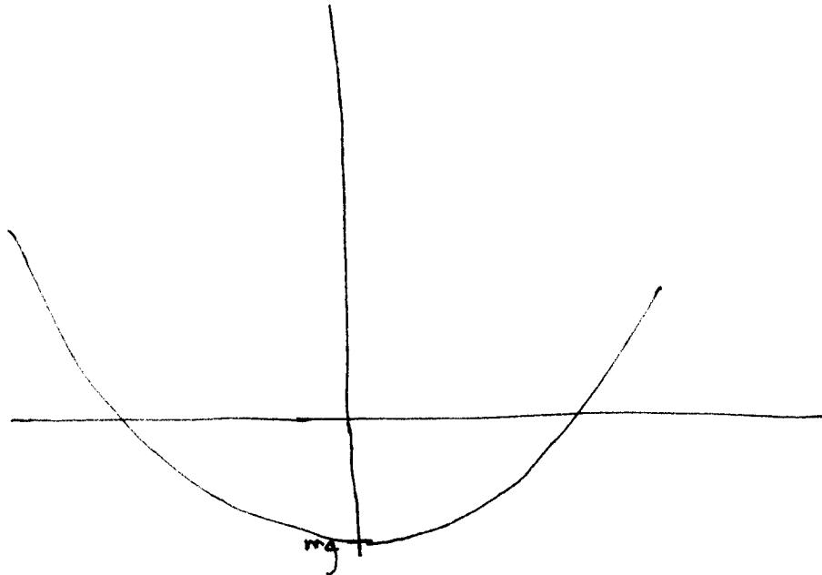
$$v^2 + \frac{c_1}{c_2} v - \frac{mg}{c_2} = 0$$
