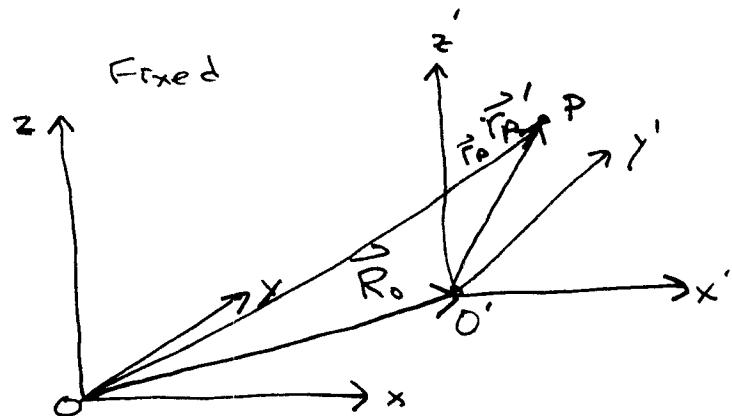
Let  $\vec{R}_0$  be a vector from the origin of the fixed coordinate system to origin of the moving coordinate system.
