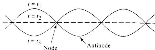
Figure 11.6.3 A standing sinusoidal wave.
