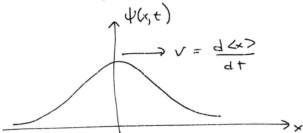
The speed of the average location of the wave  $\langle x \rangle$  is called the group velocity,
